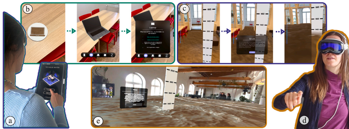
Fig. 1. (a) Outside view of the AR tablet-based prototype in the start screen. (b) screenshots of the AR objects element and (c) of the AR simulation element. (d) shows the outside view of the MR prototype, and (e) the inside view of the MR simulation element at 120 cm water level.
